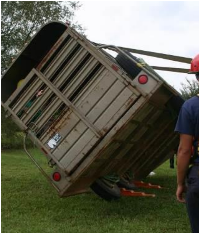
Fig. 31.1: Righting capsized trailers requires knowledge of how they balance and can be controlled without continuing to roll in a 180 degree flip. Usually animals are extricated before the capsized trailer is righted.
