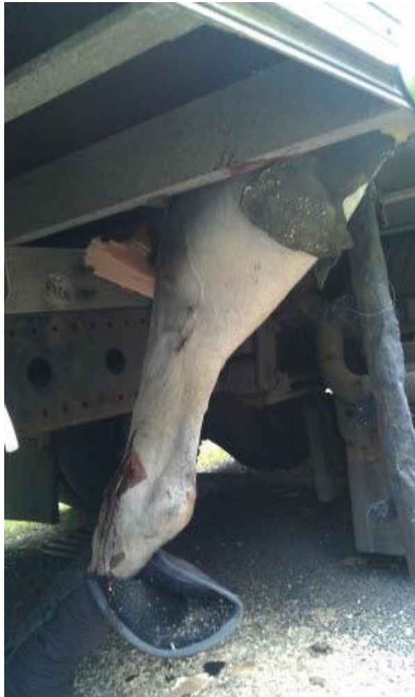
Fig. 15.4: Horses and cattle falling through new (unattached) or poorly maintained flooring are not uncommon. Wood in particular is subject to failure due to rot and should be replaced at a minimum every 10 years, or sooner if there is indication of rotting. This horse was spared greater injury by the use of leg wraps on the lower legs.
