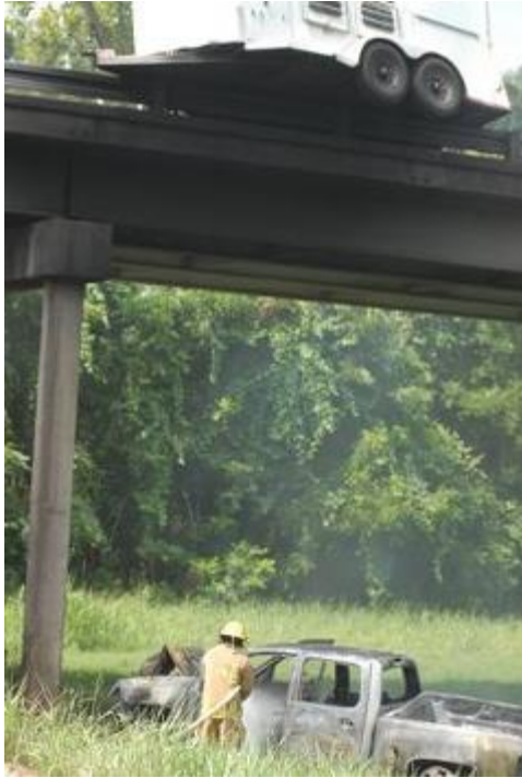
Fig. 22.4: Trailer sway sent this rig ricocheting from one guardrail to another across the road. The trailer, carrying two horses, detached to hang over the side of the bridge. The pickup plunged thirty feet below. The 17-year old driver and her young sister escaped before the truck burst into flames.
