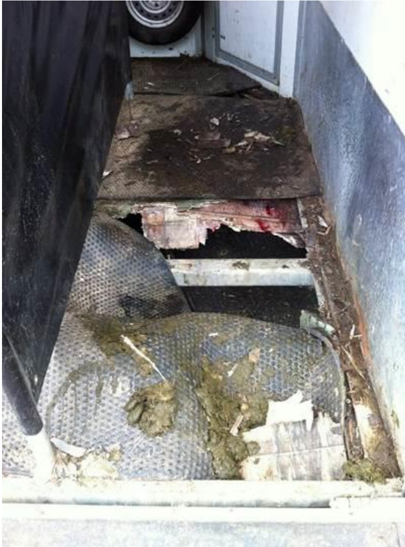
Fig. 15.2: Insubstantial flooring, widely spaced cross-members, and possibly lack of maintenance contributed to the death of the horse.
