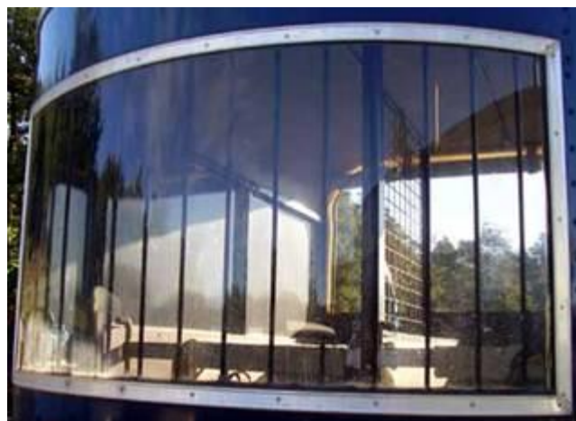
Fig. 21.4: Horses orient toward light. Good lighting in a trailer is helpful for loading and working with animals inside, but large windows present numerous hazards. This window does not have structural integrity to protect against protrusion of the horse's head or hooves in collisions or even if the animal panics and attempts to leave the trailer.
