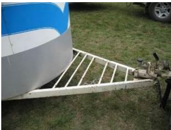
Fig. 26.2: Horses have killed themselves when a leg is caught in the open drawbar A-frame. A weight-bearing cover should be used to prevent insertion of an extremity.
