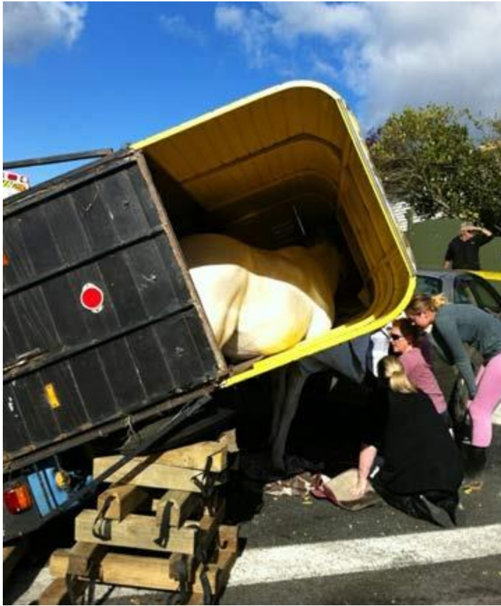
Fig. 20.2: The thin skin of most horse trailers cannot contain a hoof or head during an incident. In this case, the horse's front legs went through. Emergency responders are attempting to discern an extrication method while the owner, in a very unsafe position, soothes the horse.
