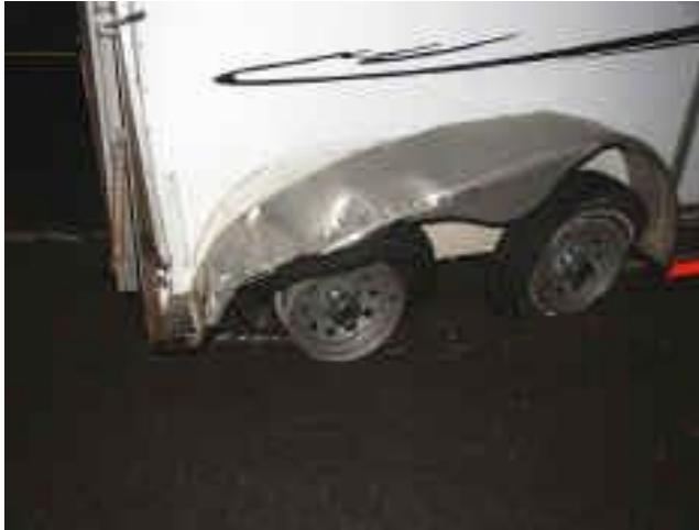
Fig. 27.3: A blown tire jackknifed the trailer, causing the tow vehicle to lose control and another truck to overturn in an avoidance maneuver.
