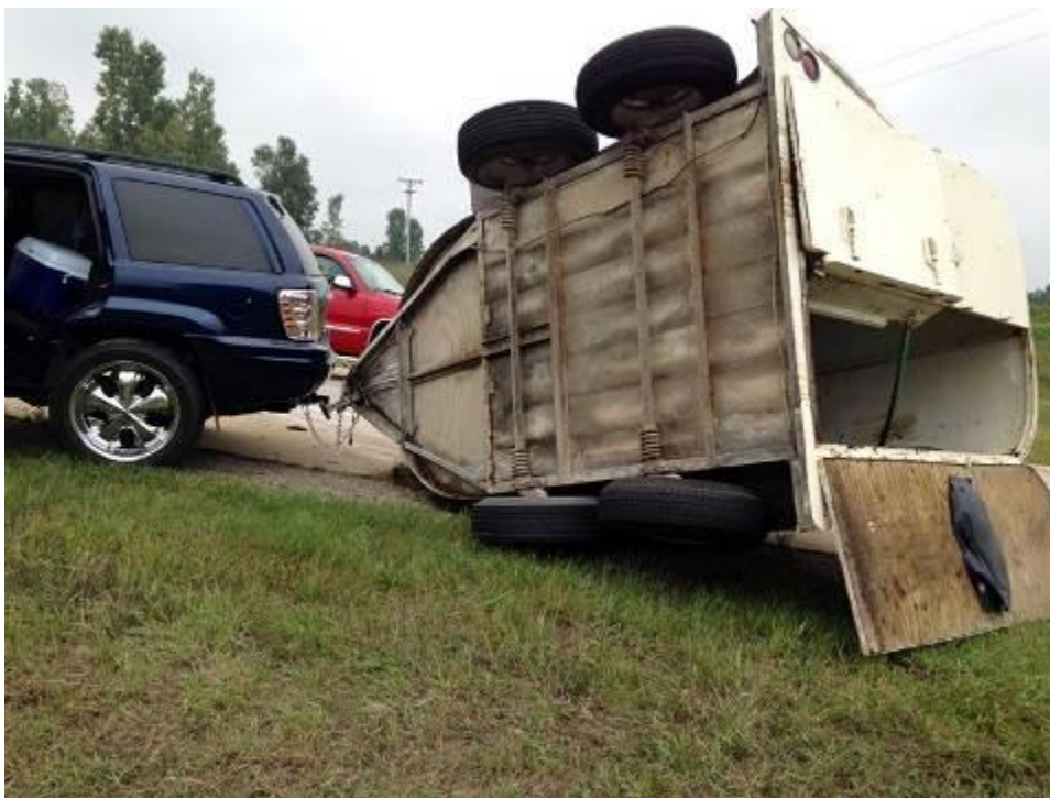
Fig. 31.3: A mismatch between trailer and tow vehicle caused this overturn. The owner insisted on the correctness of the rig. Note the plywood fore floor which would not support a horse, and the unprotected wiring.
