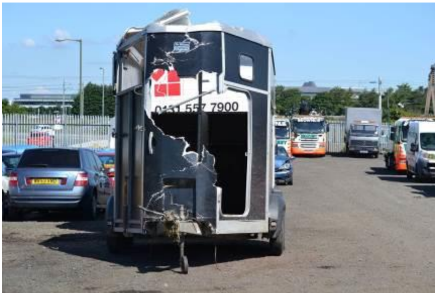
Fig. 30.3: The two-horse trailer, crashed with two horses aboard when the detachable tow bar came loose, is recovered as a write-off. Gratifyingly, the show horses survived the incident.
