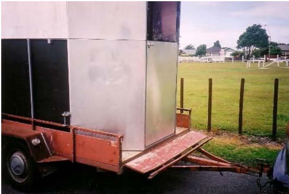
Fig. 6.2: There appears to be a window in the front of this makeshift trailer which could entice the horse to lunge through it. If it is open, it does nothing to shield the horse from exhaust or the elements.
