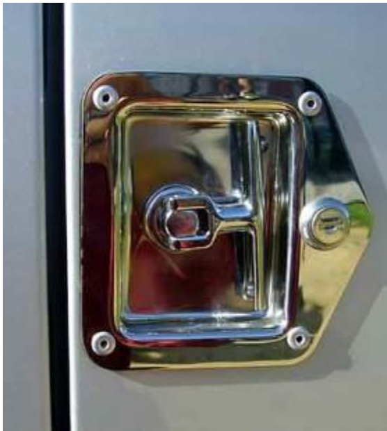
Fig. 18.8: Wherever possible, latches should be recessed or otherwise protected from injuring horses or humans.
