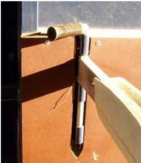
Fig. 18.4: Breast bar pins like this, too long and too sharp, are known to penetrate jugular veins, get caught on halters or lead ropes, and cause other injuries. Pins should have a safety pin through the bottom to prevent removal until warranted. Chest bars are very difficult to remove with the weight of a horse on top of them, and improved designs to facilitate removal have been slow.
