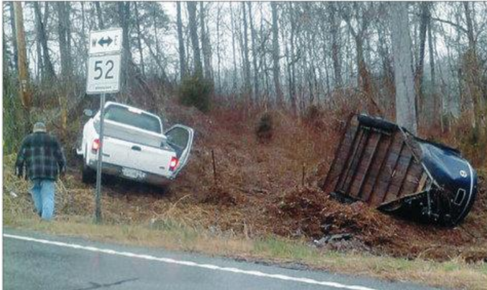
Fig. 5.9: Hitch separation followed an undescribed impact, causing the trailer to detach from the Ford F-150 and roll. A horse had to be extracted and is said to have survived. Although probably caused by incorrect hitching, this does happen in cases of hitch failure.
