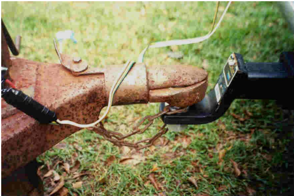
Fig. I.9: This trailer was driven 20 miles with inadequate chains, cheap wiring set-up, and unsecured latch on the “bull dog” bumper pull type coupler. However, the ball is adequately secured to the mount and the mount is secured to the receiver.
