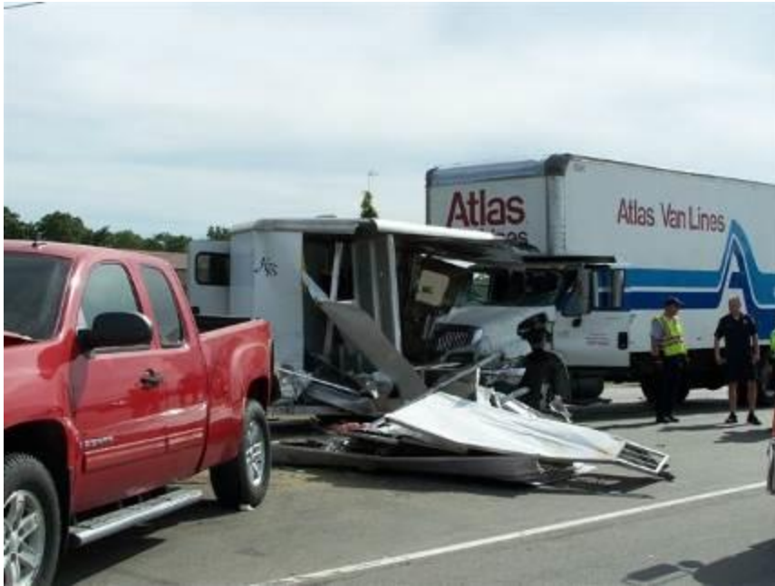
Fig. 20.6: A moving van rear ended this trailer, pushing the tow vehicle, a pickup, into a third vehicle. Only two manufacturers the committee could locate have conducted any citeable testing to determine safer ways to protect the horse from this type of impact.
