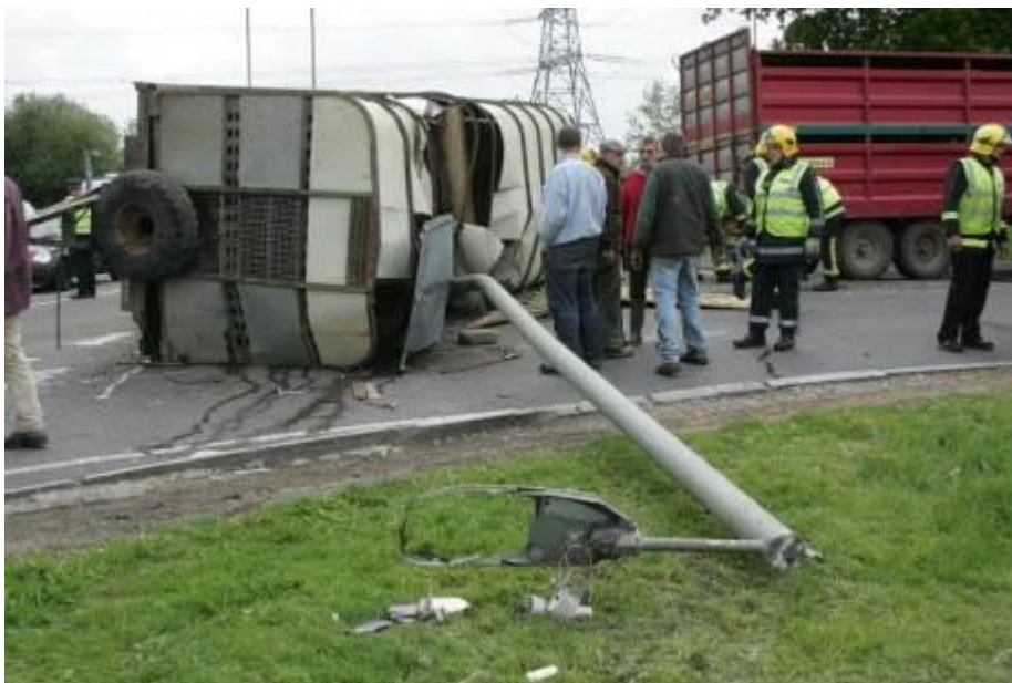
Fig. 31.5: Stock trailers and trucks are especially susceptible to tipping on roundabouts, even at slow speeds. This stock trailer was carrying sheep.
