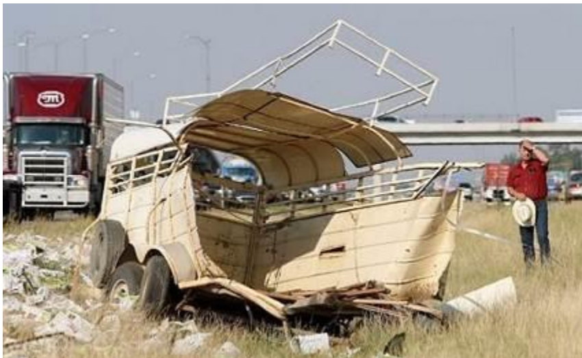
Fig. 4.4: While loaded with newspapers at the time, hitch failure sent this trailer into the median. The impact caused the trailer to rip in half. Although rarer than improper hitching, hitch installation failure does occur when the bolts work loose, pins are lost or break, or welds fail.
