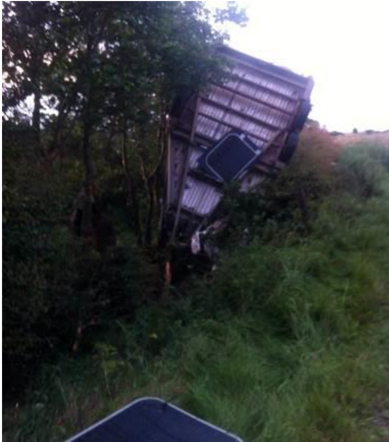
Fig. 30.2: This two-horse trailer was sent careening when the detachable (not bolted to the tow vehicle frame) tow bar failed. Numerous reports of this type of hitch failure have demolished horse and pony trailers.
