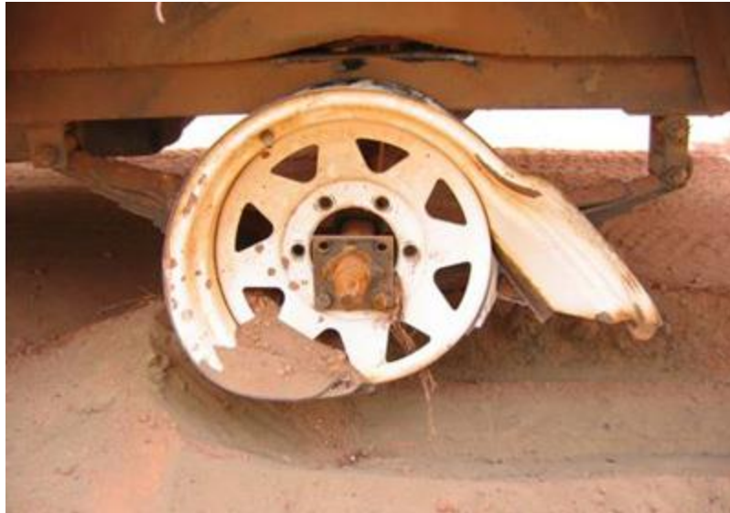
Fig. 36.1: Bearings too small for the load or wheel or not replaced with fresh grease on a regular basis whether or not the trailer is used, cause wheel failure and sometimes fires.
