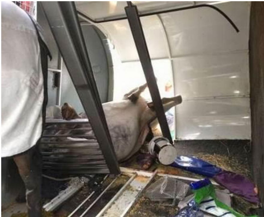
Fig. 5.16: This is the interior of Fig. 5.15. The trailer, a typical Australian slantload where the horses are standing with their noses away from the crown of the road (which is incorrect — they should be slanted the other way as Australians drive on the left) has tipped on its side. The horse was thrown forward through the "picture window," with its head exposed and legs entrapped.
