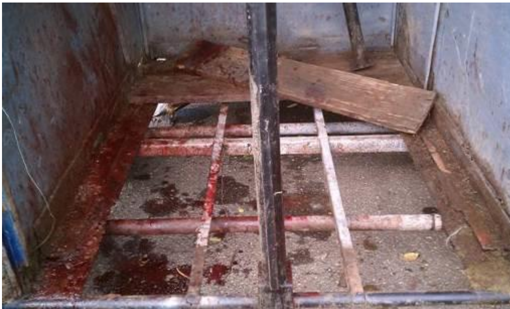
Fig. 15.1: Minimal support over the axles and no attempt to attach the floorboards to the frame have resulted in both horses dragged after falling through the floor. Both were euthanized. Photo by Milton Fire Dept., GA
