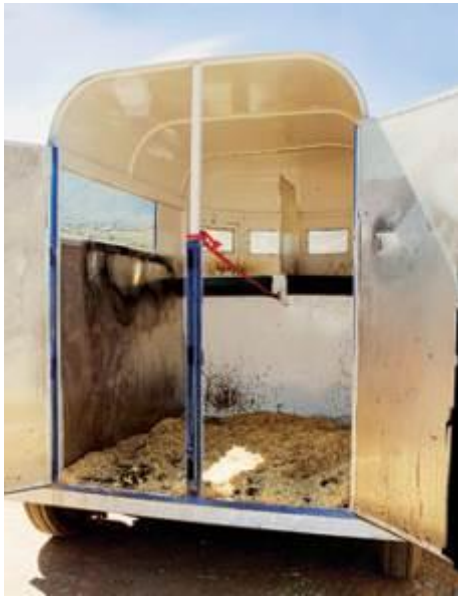
Fig. 4.1: A front panel, rear sides and a dent high in the rear door bear marks typical of a horse's attempts to retain its balance during transport.
