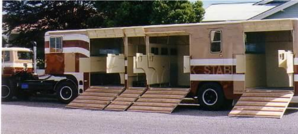
Fig. 17.7: Wide loading ramps in this rear facing van encourage easier loading. The featureless rear of the stalls leaves no butt bar to trap a horse. Ramps are shallower angled on most conventional two-horse trailer transport.
