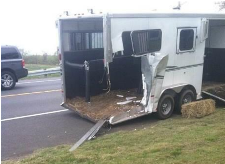
Fig. 25.11: This driver was stopped on a two-lane highway, waiting for traffic to clear to make a right hand turn when struck by a truck. The horse escaped unharmed according to initial examination, but the results demonstrate the need for stronger framing, multiple exits, and improved reflective markings.
