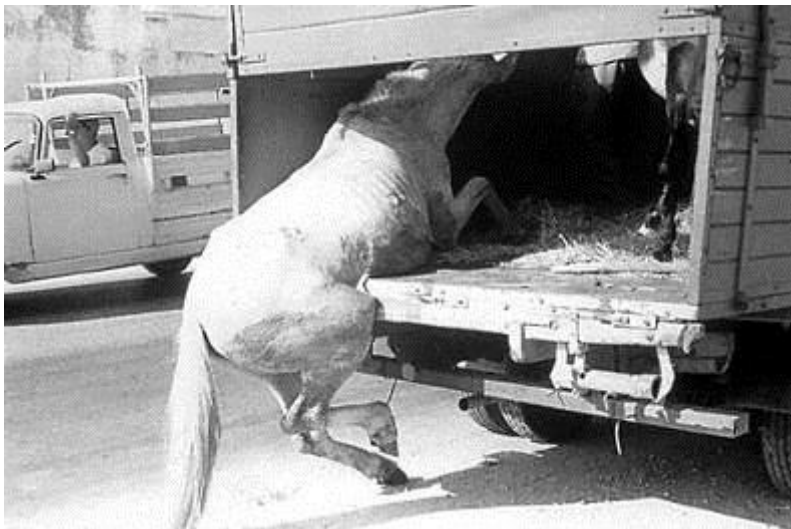
Fig. 19.1: Loaded parallel to the direction of travel, this horse is unable to retain its balance, leaned on the rear panels and is dragged because it is still tied to the van's halter ring.
