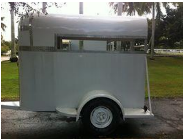
Fig. 3.4: Sold as new in 2014, this trailer needs rear side and front side lights and reflex reflectors to conform to the National Highway Traffic Safety Administration rules for conspicuity. Over 80" wide, the trailer would also require rear clearance and identification lamps and front clearance lamps.
