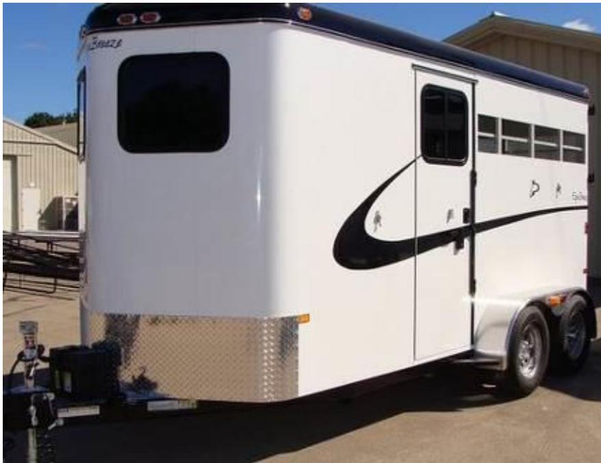
Fig. 5.11: This trailer's side vents are placed higher to discourage entrapment of a kicking horse's hoof or legs.
