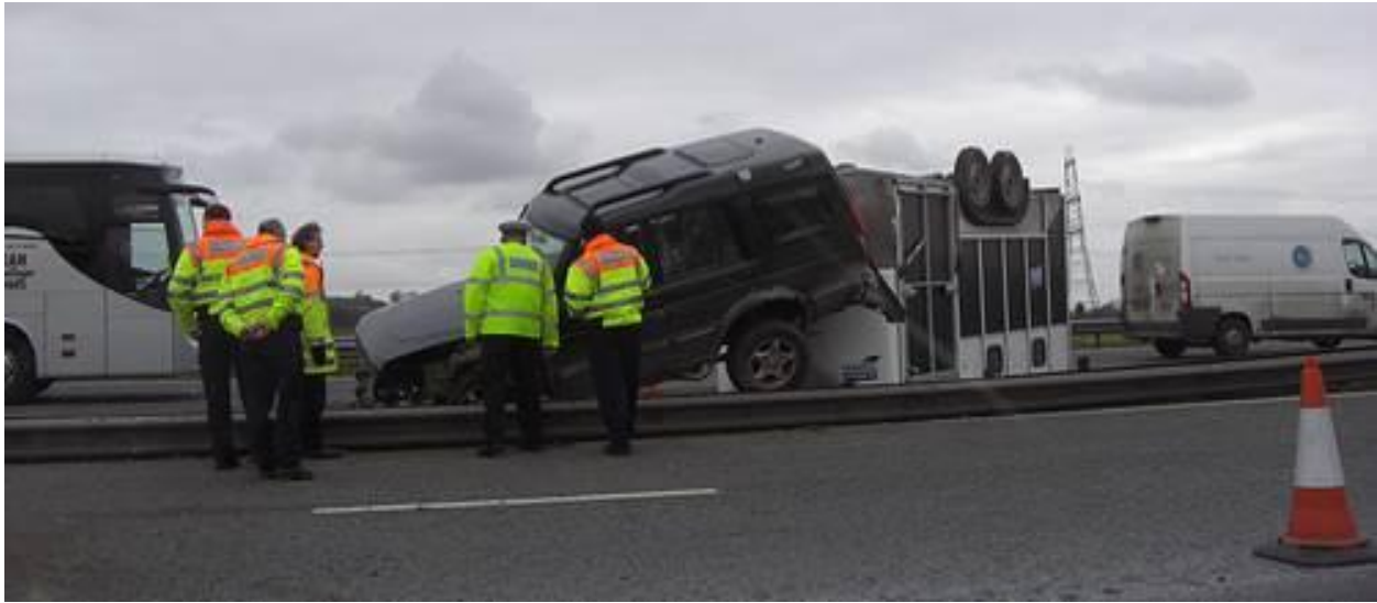
Fig. 32.2: An unsuitable tow vehicle together with a soft suspension can lead to loss of control of the rig. Sway bars are said to be unnecessary if the rig and trailer are properly matched, but very high wind conditions could mandate their use.
