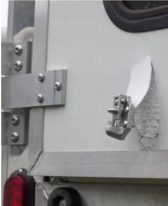
Fig. 3.7: This top door closes above a rear ramp. The door holder is screwed into a .04 (or thinner) aluminum sheet with polystyrene "sandwiched" between a similar inside sheet. There is no added support or material to prevent the self-tapping metal screw from pulling out. This is a common wall and door construction for horse trailers.
