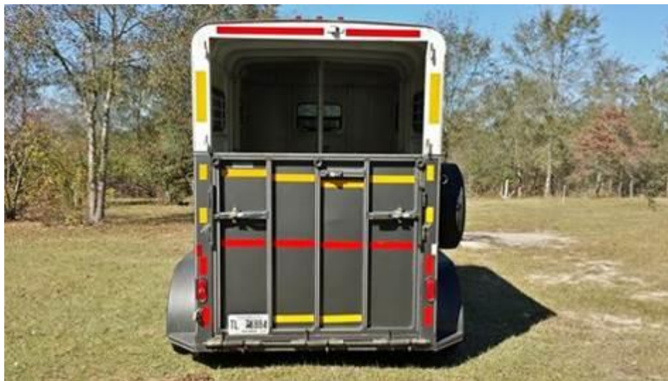
Fig 35.5: Reflective tape added to the upper sides and top of the trailer increase its chances of being detected by vehicles behind an immediately following vehicle.
