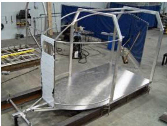
Fig. 25.15: A rollcage to field ambulance specifications and one-piece floor with the same weight bearing strength throughout contains horses within the trailer in the event of a rollover, collision, or dislodged breast bar.
