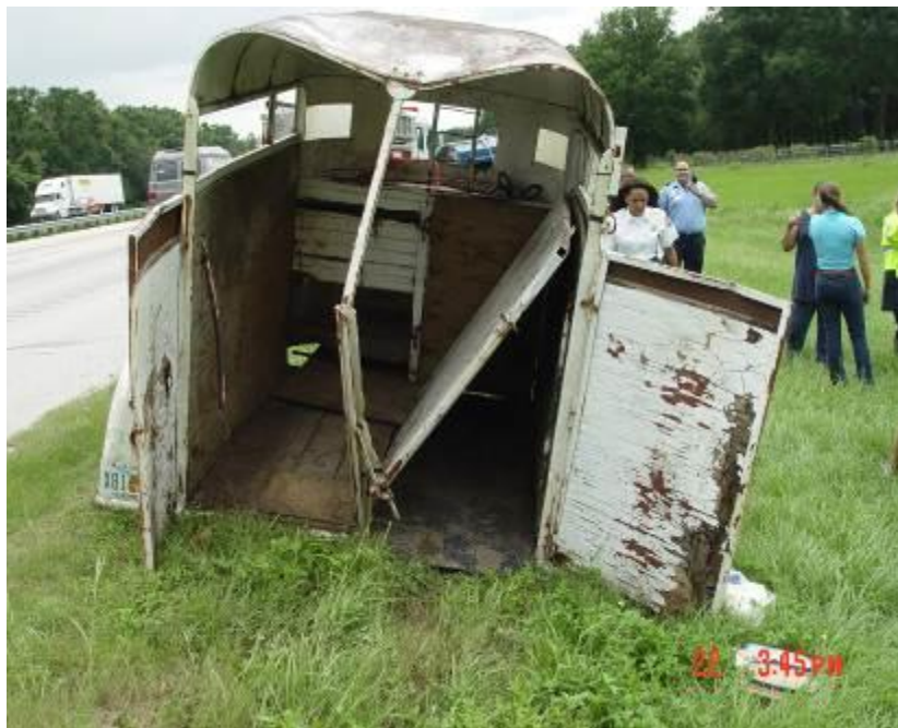
Fig. I.20: Both horses were ejected from this straight load and had to be euthanized. Mangers are in front of the horses. The partition has collapsed. The axles failed and wheels fell off. Poorly maintained trailers are commonly involved in these types of accidents.
