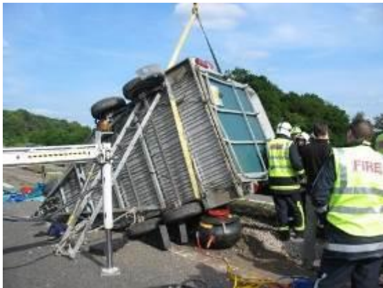
Fig. 3.6: Trailers are susceptible to overturning when overtaking, hitting an obstacle in the road, heavy or uneven braking, or swerving to avoid a collision. This trailer overturned in a roundabout when the driver had to brake to avoid another vehicle.
