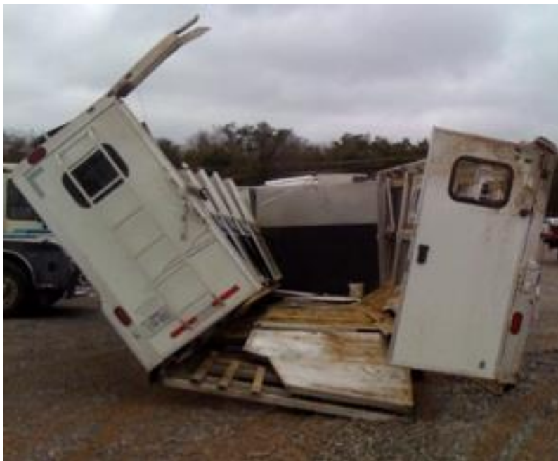
Fig. 25.5: This large trailer split open on impact, exposing the horses within. This indicates very poor construction providing no structural integrity.
