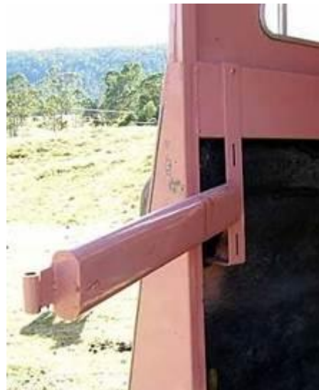
Fig. 18.5: This rump or butt bar is "as narrow as a shoelace" and offers scant support to a horse's weight if the horse pushes on it. It cannot be swung completely out of the way and presents a fixed hazard to both people and horses when loading or unloading.
