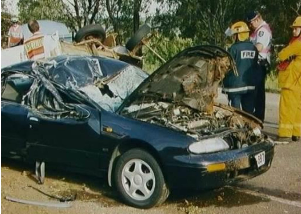
Fig. 22.1: At high or low speeds, trailers can overturn due to hitch failure, loss of control on ice, hard braking, or wind gust. On the highway, other vehicles become potential landing zones for this type of incident.
