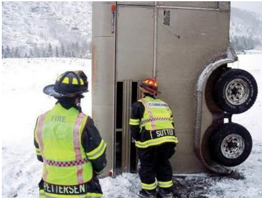
Fig. 22.3: Responders approach this detached, upended trailer. A properly hitched trailer does not come detached. Electronic brake controls might have prevented this incident.
