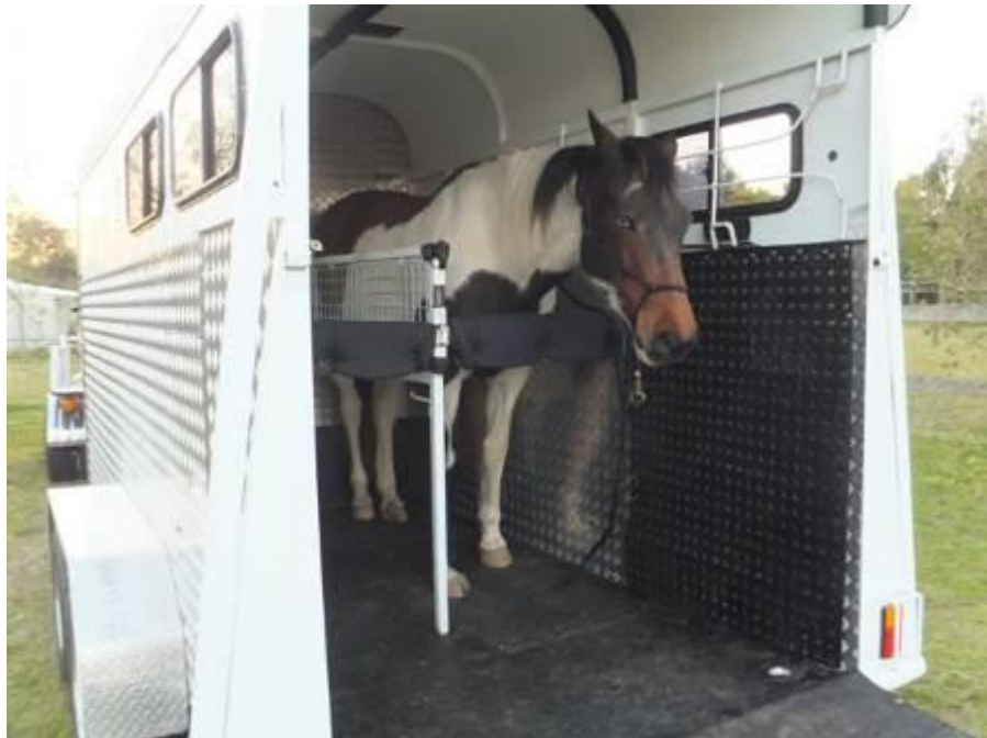
Fig. 11.9: This horse's weight in a rear face position is located between the axles, at the point of least rotation. Its thoracic sling is free to act as gimbals, which tends to make the horse more comfortable in transport.
