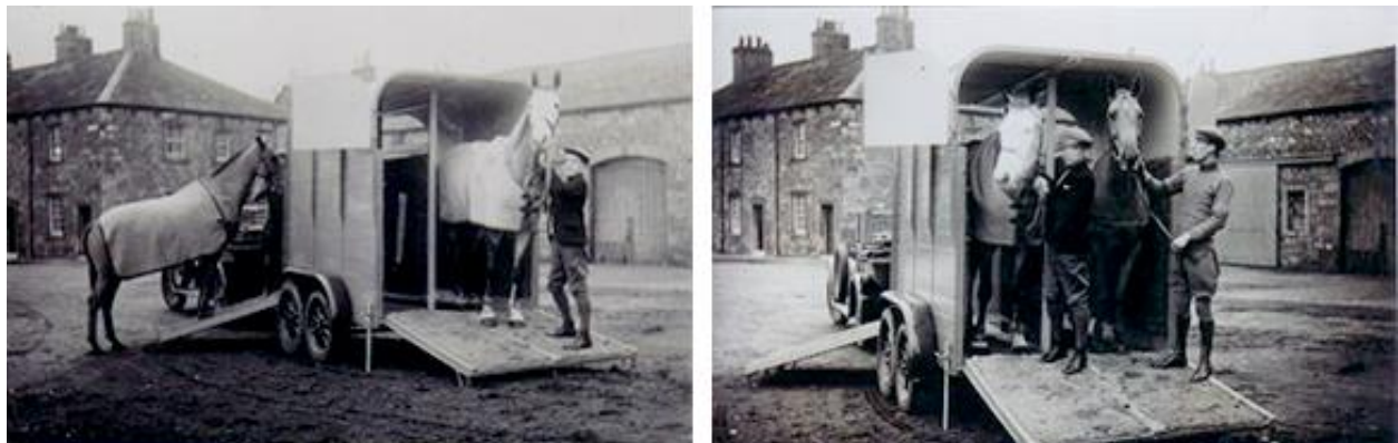
Fig. 11.2: This 1930s trailer by Rice loaded the horse from the front of the trailer to face away from the direction of travel. This method, re-popularized today, places the horse near the hitch and possible injury if there was an incident. It also did not eliminate the presence of a handler within the trailer.
