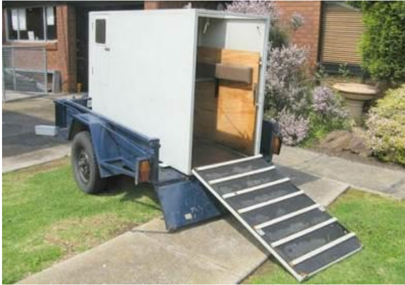
Fig. 4.3: Single-axle garden trailers are not appropriate for hauling live weight. There are numerous examples of tragic accidents with this type of trailer.
