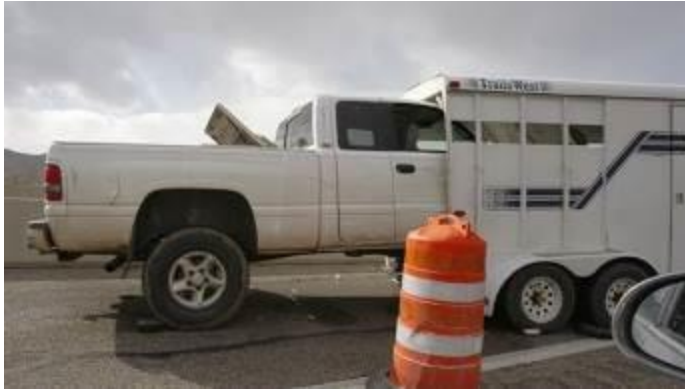
Fig. 25.10: Underride guards and better framing could protect many horse trailers from maximum intrusion when rear ended or rammed from the side. Maximum use of forward exits large enough for horses is preferred. Additionally, improved reflective provisions would allow following drivers to see the rig in the first place.
