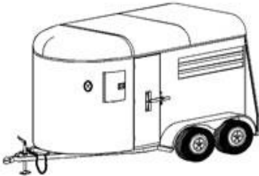
Fig. I.19: In this example, a tag along trailer in which the horses are loaded and transported facing the direction of travel. May also be gooseneck or 5 th wheel versions.
