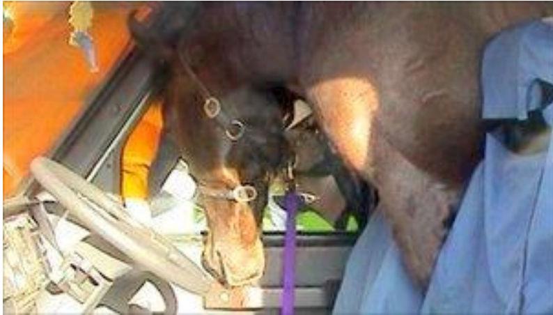
Fig. 25.8: This horse broke through into the cab of the van, trapping the jockey. Manufacturers of horse trailers and vans must strengthen the bulkhead against such events.
