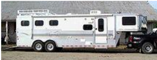
Fig. I.5: A gooseneck trailer hitched into the bed of a pick up.
