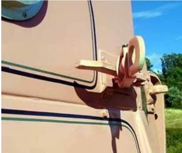
Fig. 18.6: This projecting latch presents a hazard to passersby and horses.
