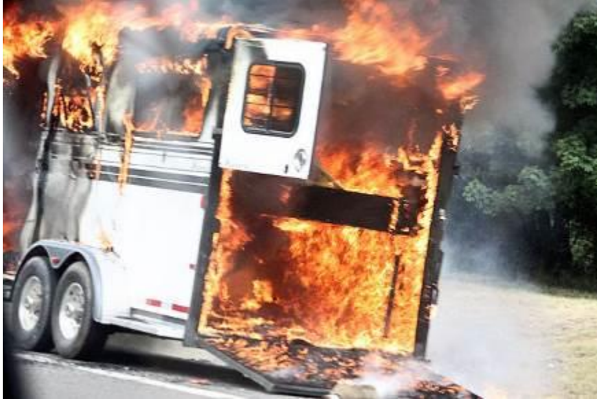
Fig. 3.2: Electrical shorts, gasoline or propane leaks, hay, flying cigarettes, or other causes can easily ignite some cargo or the trailer. All release toxic gases. Fortunately, no horses were in this trailer.
