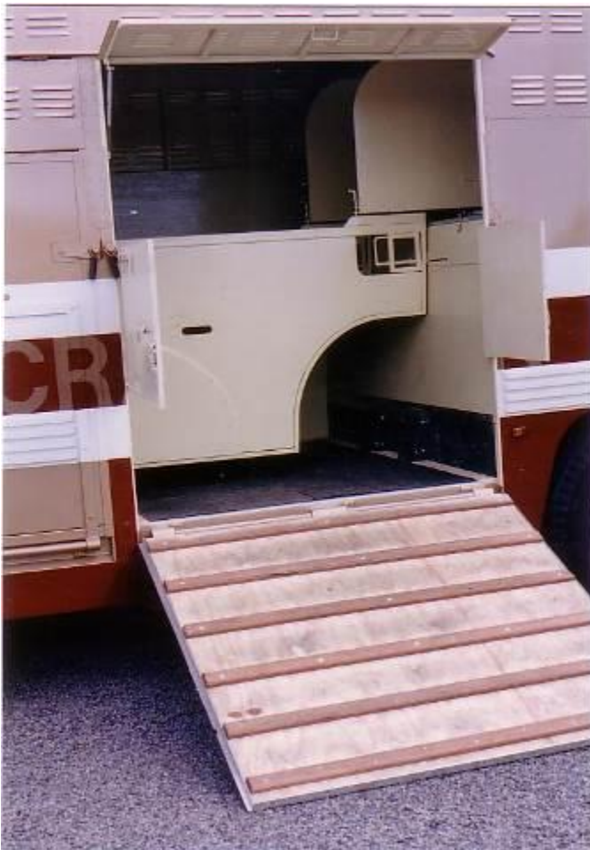
Fig. 17.8: Cut-away partitions in this thirteen-horse rear-facing van allow greater air circulation. Solid head dividers are better replaced by barred dividers, not only for air circulation, but horses travel more quietly when other horses are in view.
