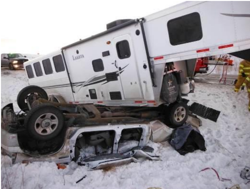
Fig. 5.1: An overturned horse trailer totaled this vehicle. It is not uncommon for trailers to land on passing vehicles when they roll.
