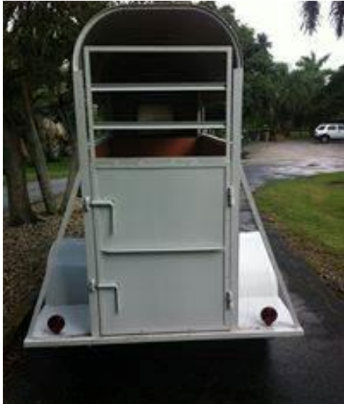
Fig. 3.3: Single-axle trailers are probably the least stable trailer in use. Place a high-centered load, like a horse in them, and the tendency to snake is increased.
