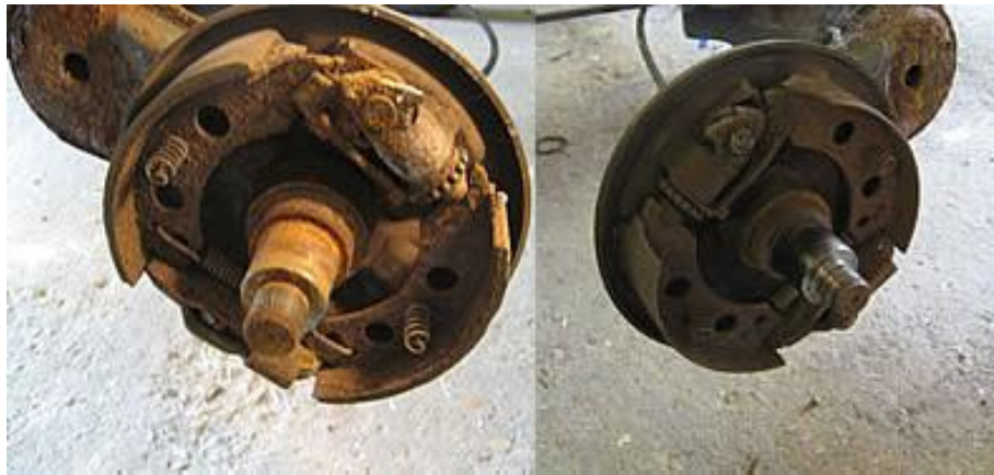
Fig. 36.3: Typical of poor trailer maintenance are inoperative, corroded, worn or poorly adjusted brakes. Haulers should be schooled in inspecting and adjusting brakes to the load.
