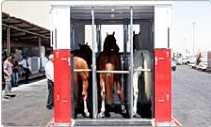
Fig. 10.6: Horses facing the direction of travel tense and seek to stabilize themselves even before this air freight stall moves off. Their hind legs are spread outside the hip joint as widely as the confines allow. This position puts strain on the stall partitions and fittings. Horses feel more comfortable and scramble less or not at all when they have freedom of movement to balance without strain.
