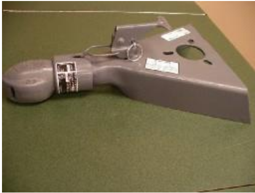
Fig. I.8: Bumper pull, AKA “tag along” coupler with safety pin in latch. This one is commonly referred to as a “bull dog” because the jaws of the hitch close around the ball, then a sliding latch closes over the jaws and is pinned in place.
