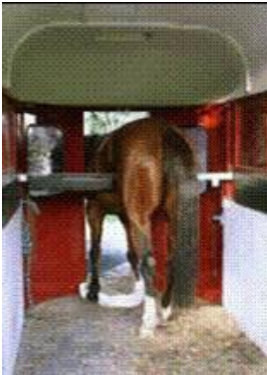
Fig. 19.2: This horse has leaped the breastbar and impaled the deck ahead of the breast bar with a hoof. Often the forward area is not built with the same support as the area that the horses stand on. This demonstrates why the entire floor should be well supported.
