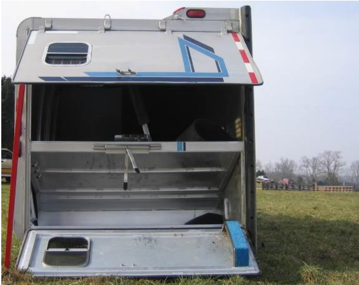
Fig. I.18: Flipped to the left, this trailer shows how permanent structurally sound components can offer challenges to accessing the animals. Once the saddle racks and the rear doors are removed, this trailer will allow safer and easier access to the animals.
