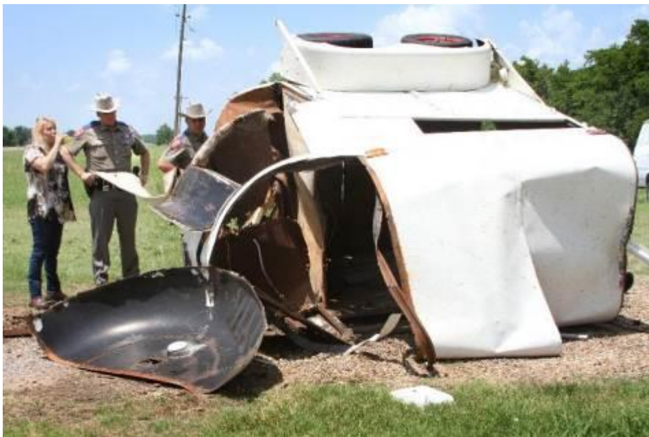
Fig. 30.1: Hitch failure (separation of the frame of the nose of the trailer from the body of the trailer) caused this overturn, leaving the horses unprotected and injured. The construction of this trailer is cheap in every way.
