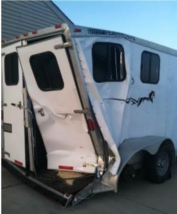
Fig. 25.13: Doors and frame diffused some of the impact, putting the horses in this rear ended trailer at less risk than in some trailers.
