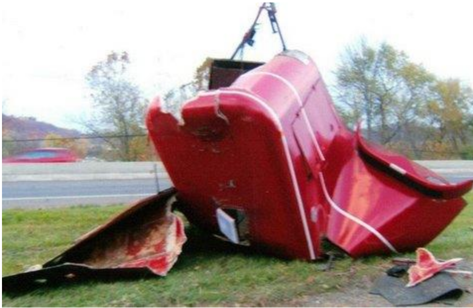
Fig. 4.5: The two horses in the trailer survived this disaster. It came unhooked from the tow vehicle. Poorly configured trailers split open when insufficient structural integrity is provided — in this case the trailer was made of fiberglass which simply peeled apart on rollover of the trailer.
