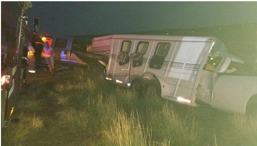
Fig. 5.2: This texting driver rear ended the horse trailer. Reinforced ramps, frames and possibly underrider guards are needed to protect horses from these frequent incidents.
