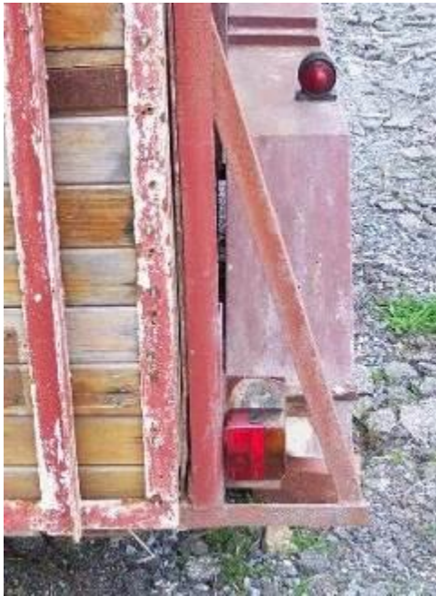
Fig. 26.1: Though not a drawbar, this is a common failing of many trailers, old and new. Their open frames and braces can trap a hoof or extremity.
