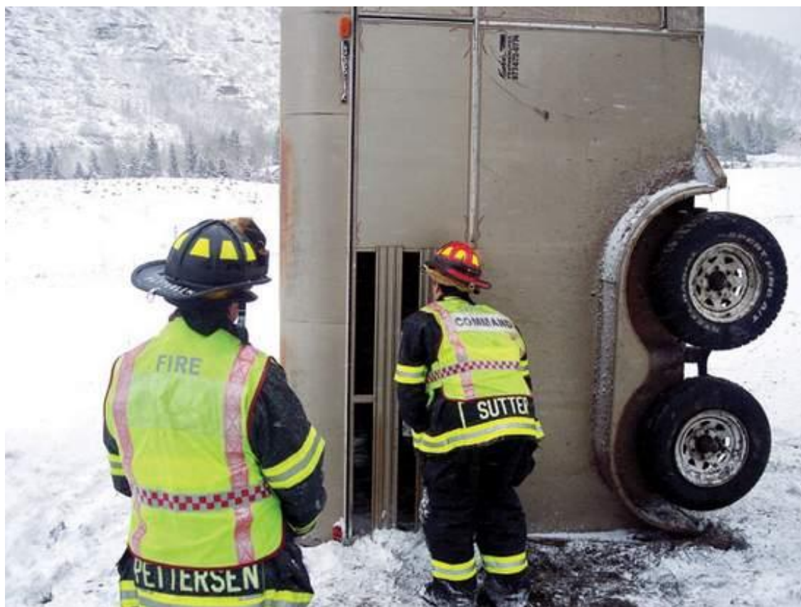
Fig. I.13: An incorrectly hitched trailer is susceptible to separation from the tow vehicle when braked too quickly or in a collision. Two horses inside, this trailer ended in a field.
