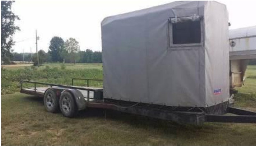
Fig. 20.1: While it meets the criteria of shelter from the elements, this canvas skin is unlikely to survive a restive horse or protect the horse during an incident.
