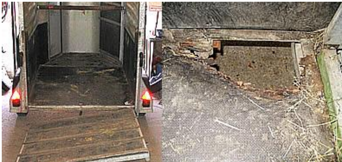
Fig. 36.2: Ramp hinges are notorious for failure. Covered by ramp skin or exposed, they collect urine, feces, and damp. Heavy matting discourages frequent removal for cleaning, drying, and inspection after each trip.
