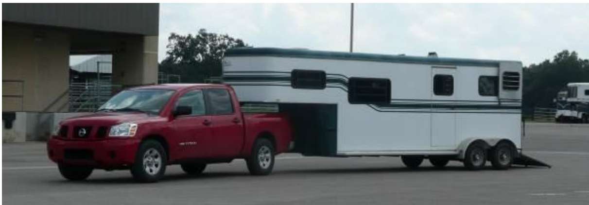
Fig. I.12: A common failing of hitches is that the trailer is not level.
