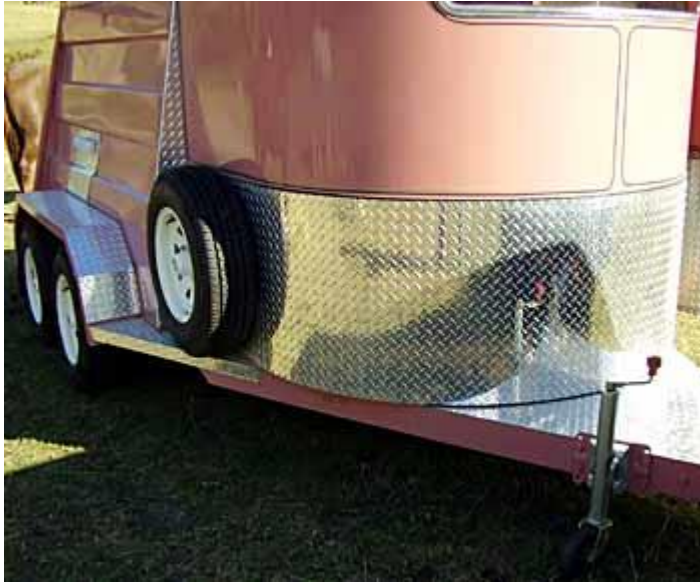
Fig. 26.3: The drawbar frame of this trailer is solid to prevent a horse from getting its leg trapped.
