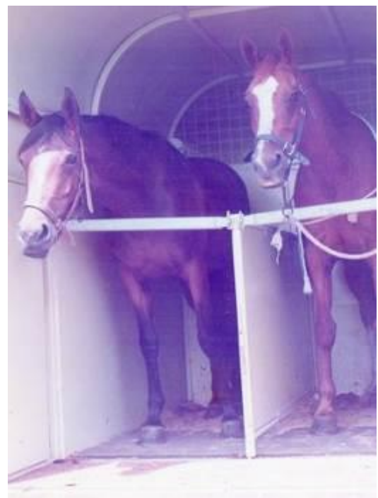
Fig. 19.5: Gypsy, on the left, is properly tied back at the withers. Copernicus is carelessly tied and could readily leap the breast bar. The partition is not quite to the floor and could trap a shod horse. The exposed bow frames are not recommended. However, there are no scramble or kick marks on the partition or sides of this early version of rear face trailer transport.
