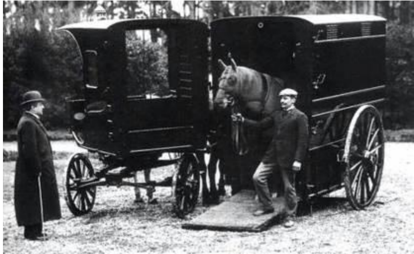
Fig. 1.6: From its inception, the practice of vanning recognized the hazards associated with reversing horses to unload. Horses may react to novel stimulus from behind or uncertain footing by jumping forward or kicking. Provision was made in many vans, including this one from 1897, to place the handler at the horse's head and unload forward from the front of the van. The team for this horse drawn van has just been unhitched and led away.
