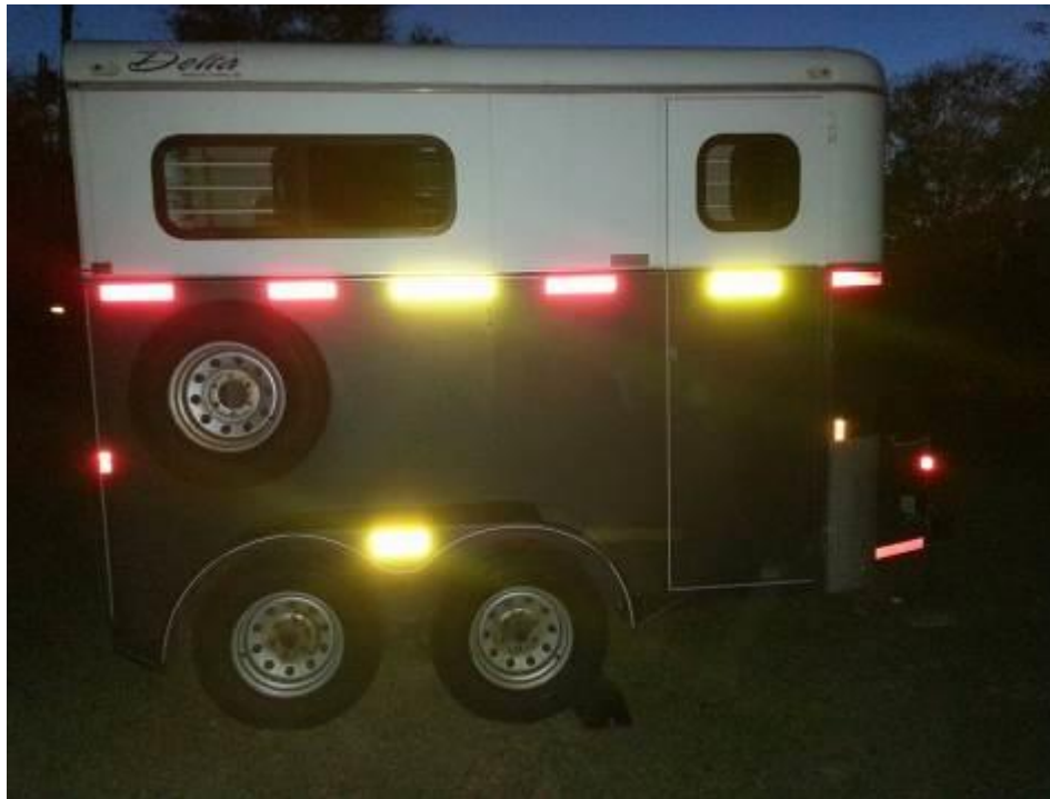
Fig 35.4: With added reflective tape, the trailer in Fig. 35.3 is now conspicuous even by a camera flash.
