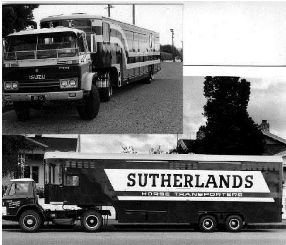
Fig. 17.6: These vans travel twelve horses facing away from the direction of travel and one parallel to the direction of travel. The latter is not recommended as horses have poor sideways balance.
