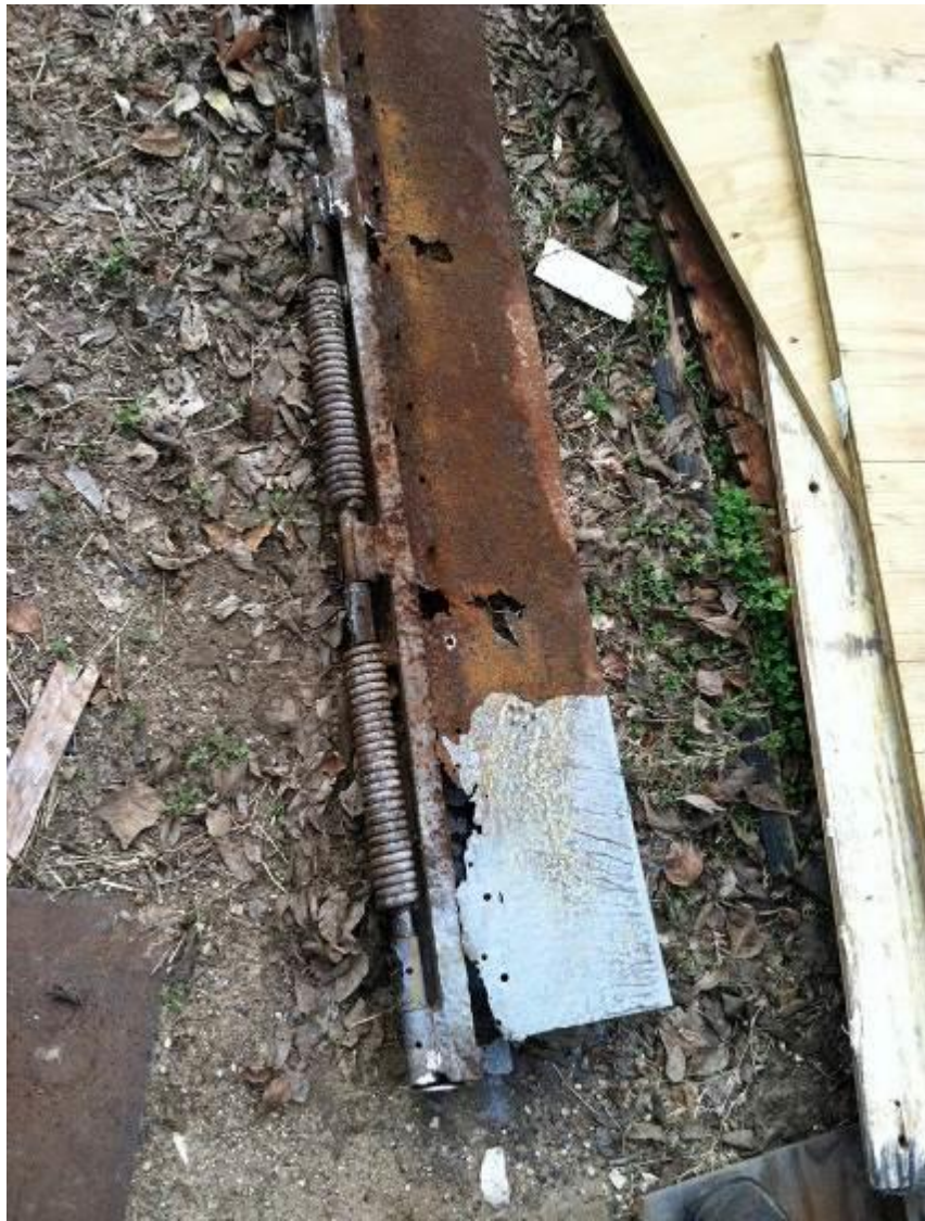
Fig. 7.3: Trailer skin wrapped around the hinge concealed the weakening of the ramp. Photo: Courtesy of J. Johnson.
