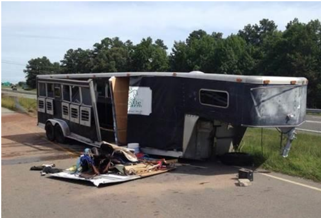
Fig. 25.6: A tire on the tow vehicle failed, despite having been inspected within the last 24 hours. Rig control was lost, the trailer came unhitched, started to roll, then landed. The impact loosened the sidewall, and four of the five horses exited through the opening. The tow vehicle rolled five times.
