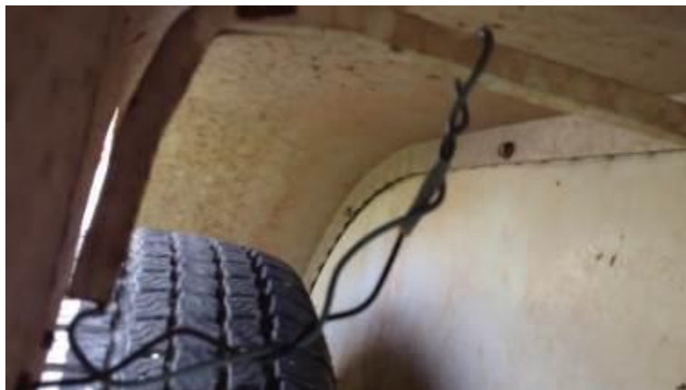
Fig. 33.1: These two entwined wires almost escaped discovery. Located in the wheel area, they will almost certainly short at some point from moisture and debris.
