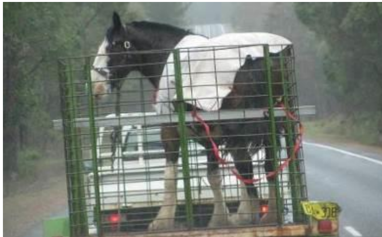
Fig. 3.5: A homemade trailer offers no containment or protection of the animal (in this case one that weighs over 1000 kilograms) from flying debris, sand, dust, cans and cigarettes thrown from passing vehicles. No test for road worthiness is currently required.
