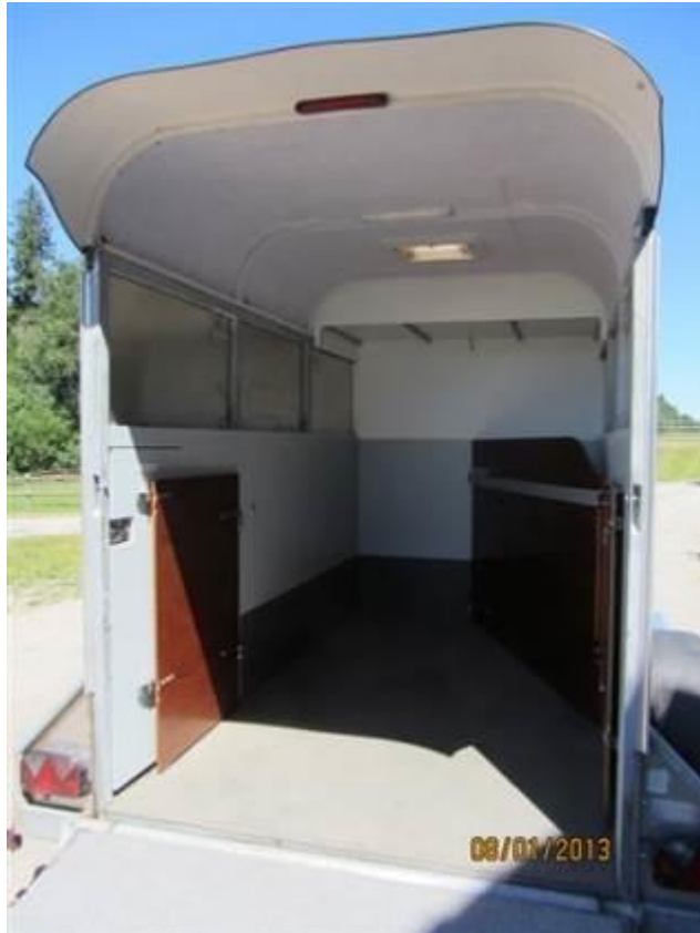
Fig. 11.11: A protected entry against possible head injuries and the elimination of activity behind it and rear restraints, reduces the chances of a loading or unloading incident. A flat white interior presents no glare.
