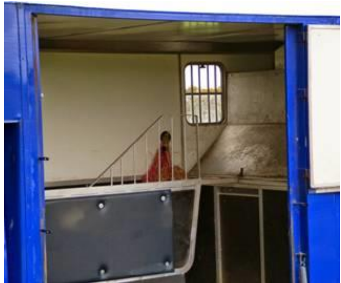
Fig. 19.9: In this rear facing trailer, poor tying practices did not prevent the horse from leaping the chest barrier. The added barrier in front of the horse is intended to discourage a leap, but is unlikely to do so. It will also prevent the horse from lowering its head to clear its respiratory system.
