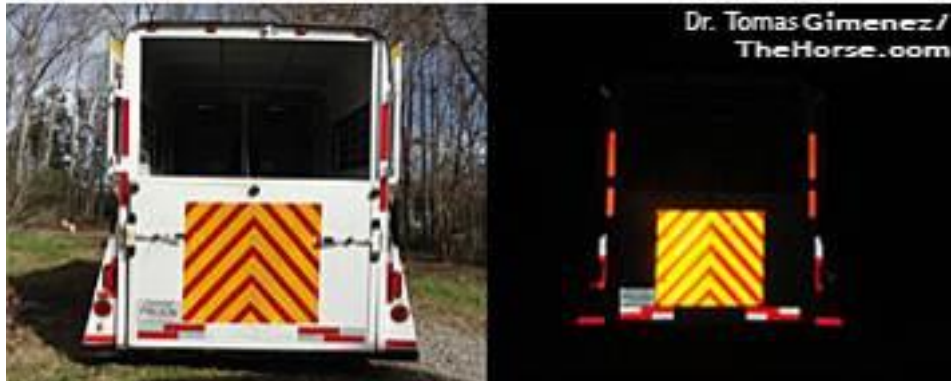
Fig. 35.1: A professional Technical Large Animal Emergency Rescue instructor owns this personal two horse trailer and has maximized its conspicuity markings. Note that even though it is a white trailer, the white is not visible in the dark when lit by following headlights.
