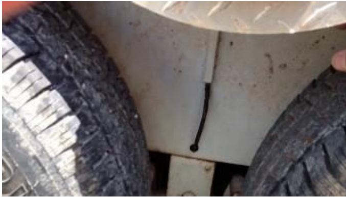
Fig. 33.2: The trailer owner has wrapped this wire with electrical tape to try to prevent moisture damage. Located between the trailer wheels, it could still be caught in a horse's pawing hoof.
