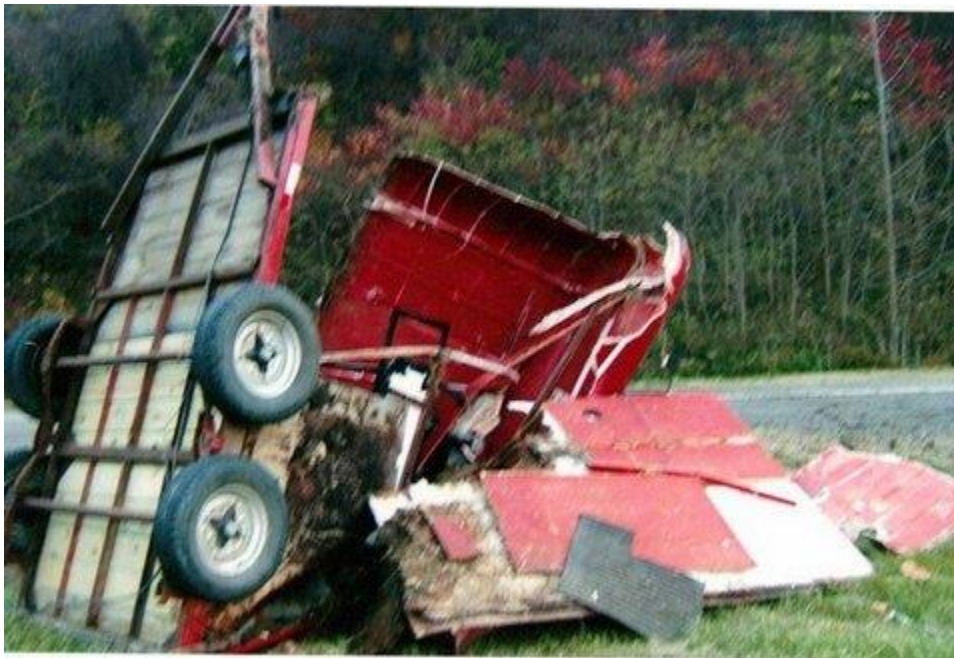
Fig. 4.6: This trailer, the same as that shown in Fig. 4.5, shows the typical angle floor frame with 1x1 tube side frame up to 1.2 meters apart with smooth fiberglass side walls. Plywood lines the inside walls. Side-to-side floor boards are not recommended, especially with only one piece of metal beneath. Other viewers suspect that the wood liner may have retained moisture, rotting the wall supports.
