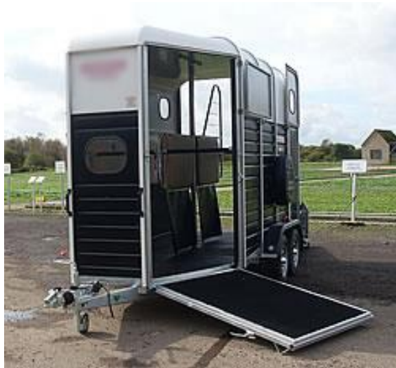
Fig. I.16: There are numerous kinds of rear-face trailer. In this design, the horse can get trapped in the open A-frame tongue. The people behind stand in the kicking zone. Without provision for a platform load, the entry ramp adds unnecessary weight. A similar arrangement to the one above earned the handler a broken arm when the horse crowded against the handler leading it in. Many manufacturers provide a tie-up in the wrong position, allowing the horses to leap the breast bar.
