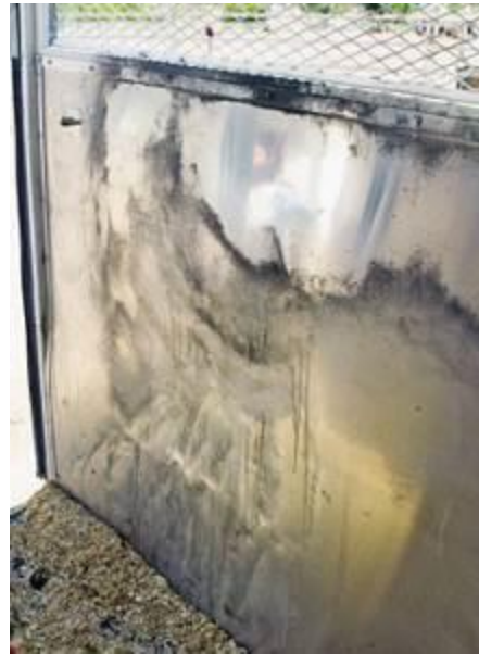
Fig. 4.2: A close-up look of the rear side of this trailer's aptly named kick board, shows the marks of a horse attempting to broaden its rear leg stance. Some trailers on the market flare the sides to accommodate these attempts, but these interior flares continue to record the horses' struggles.
