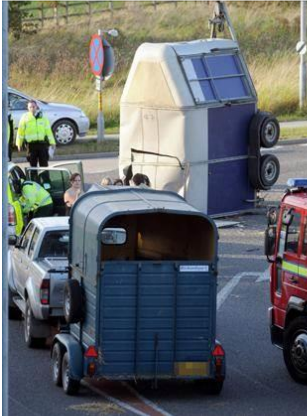
Fig. 9.7: Inadequate hitching or mismatched ball and coupler, a failed or disconnected electrical brake are among the contributors to incidents landing trailers on their rear doors.
