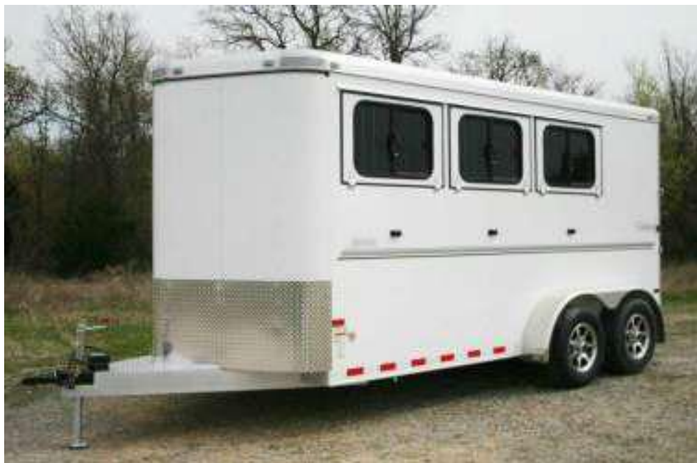
Fig. I.7: Sold as a light-weight 2-4 horse bumper pull, this trailer cannot be safely towed by anything less than a 3,500i dual rear wheel truck.
