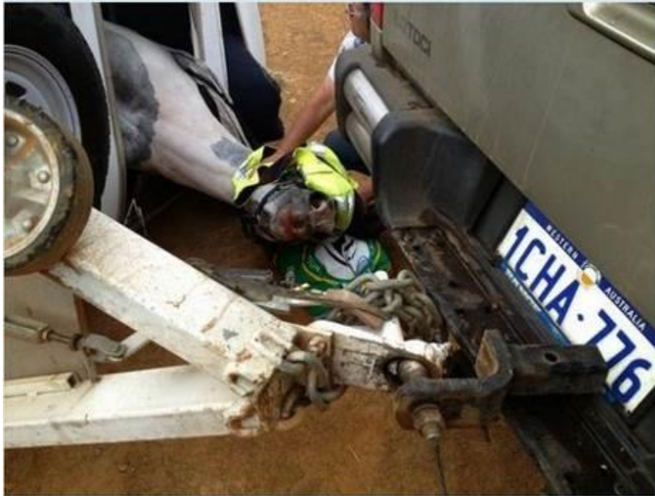
Fig. 5.15: Hitch separation (note the lack of the hitch pin) on a gravelled road caused this trailer to overturn, although the chains maintained its attachment to the towing vehicle. The horse is ejected partly through the front of the trailer's "picture window," even though the driver was proceeding slowly.
