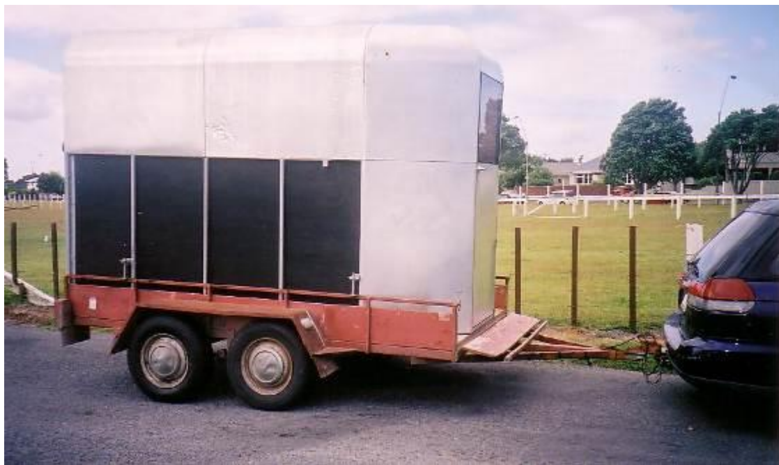
Fig. 6.1: A simple box bolted onto a garden trailer at four points passes for a horse trailer.
