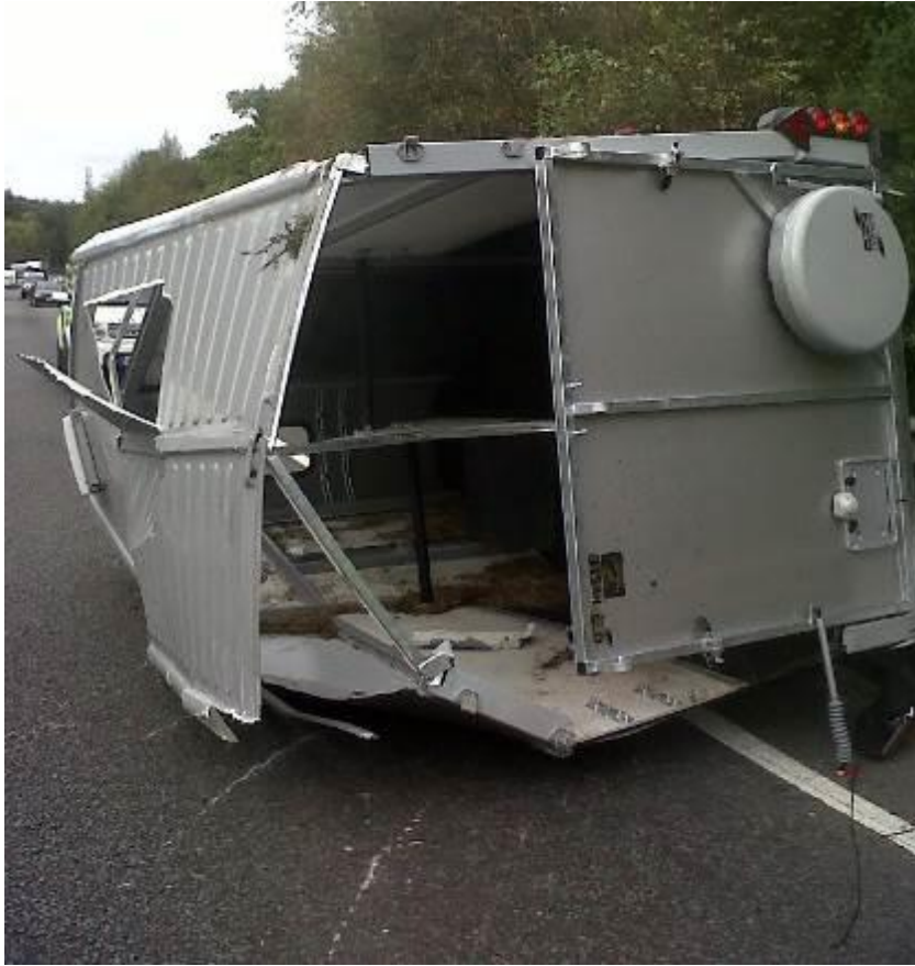
Fig. 25.4: Less than a week old, this aluminum trailer has overturned. The weakness of the trailer/float skin, frame and bows can hinder rescuers from using support cribbing to stabilize the trailer and requires careful evaluation of strut or cribbing placement.
