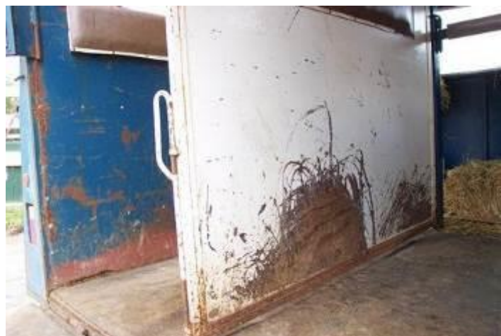
Fig. 10.5: Partitions and kick boards in conventional floats record the efforts of the horse to remain upright.
