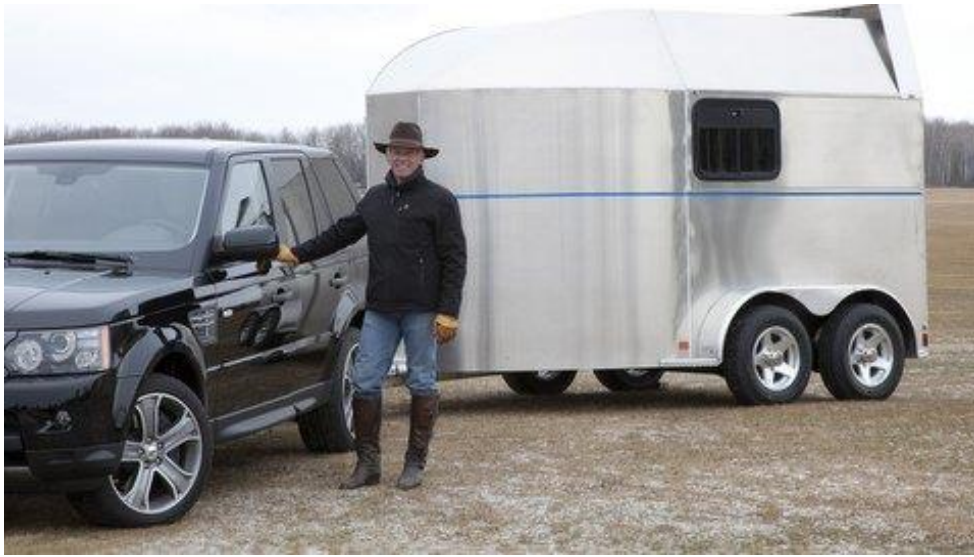
Fig. 20.7: Committee member J. Sigurdson stands with one of his firm's unibody horse trailers. Built to field ambulance standards, its skin of up to 3mm thickness of 5052 H32 aluminum allows a horse to safely stand on the roof without penetrating.
